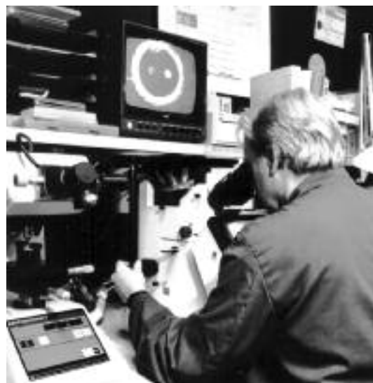
A lab service technician uses a metallurgical microscope to examine the microstructure of the metallic components in Watlow's mineral insulated metal sheathed cable, XACTPAK.
